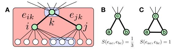
Figure 1: (**A**) The similarity measure  $S(e_{ik}, e_{jk})$  between edges  $e_{ik}$  and  $e_{jk}$  sharing node k. For this example,  $|n_+(i) \cup n_+(j)| = 12$  and  $|n_+(i) \cap n_+(j)| = 4$ , giving S = 1/3. Two simple cases: (**B**) an isolated  $(k_a = k_b = 1)$ , connected triple (a, c, b) has S = 1/3, while (**C**) an isolated triangle has S = 1.
